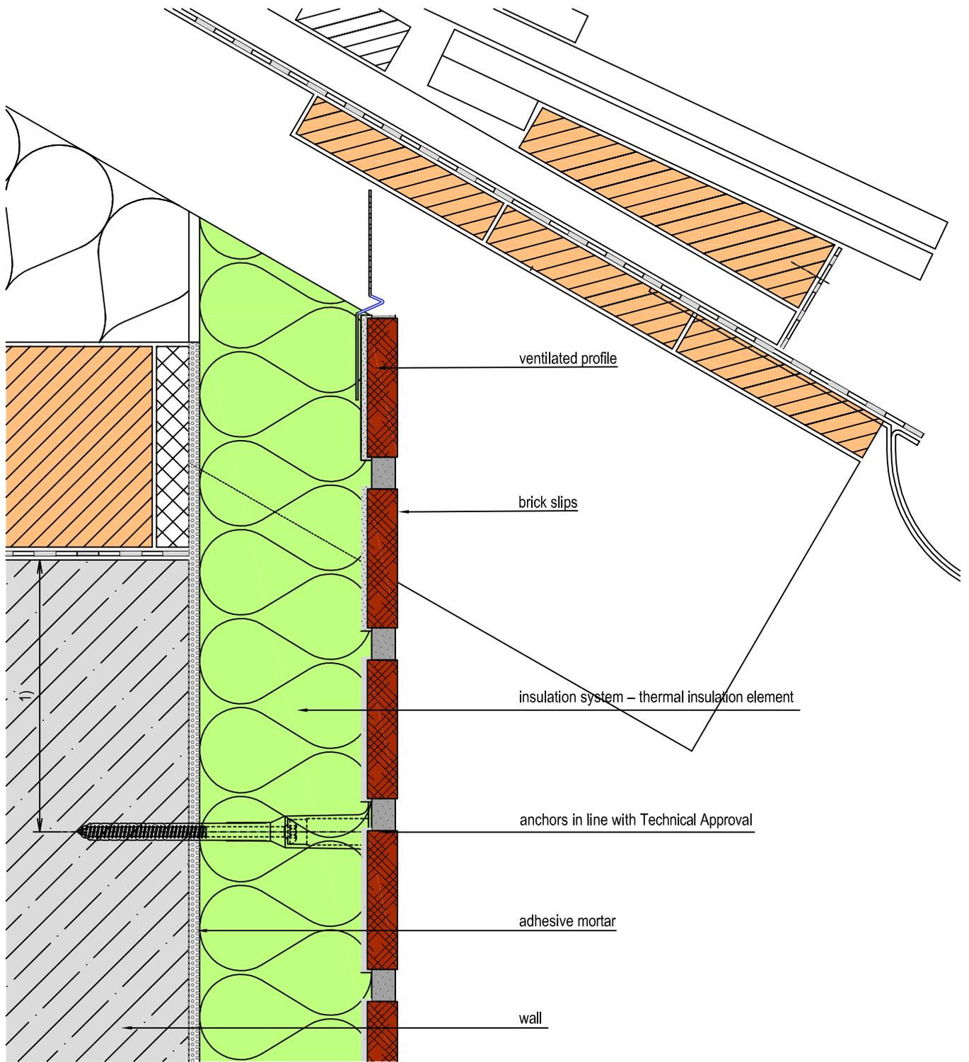
1)  $C_{min}$  anchors in line with Technical Approval
