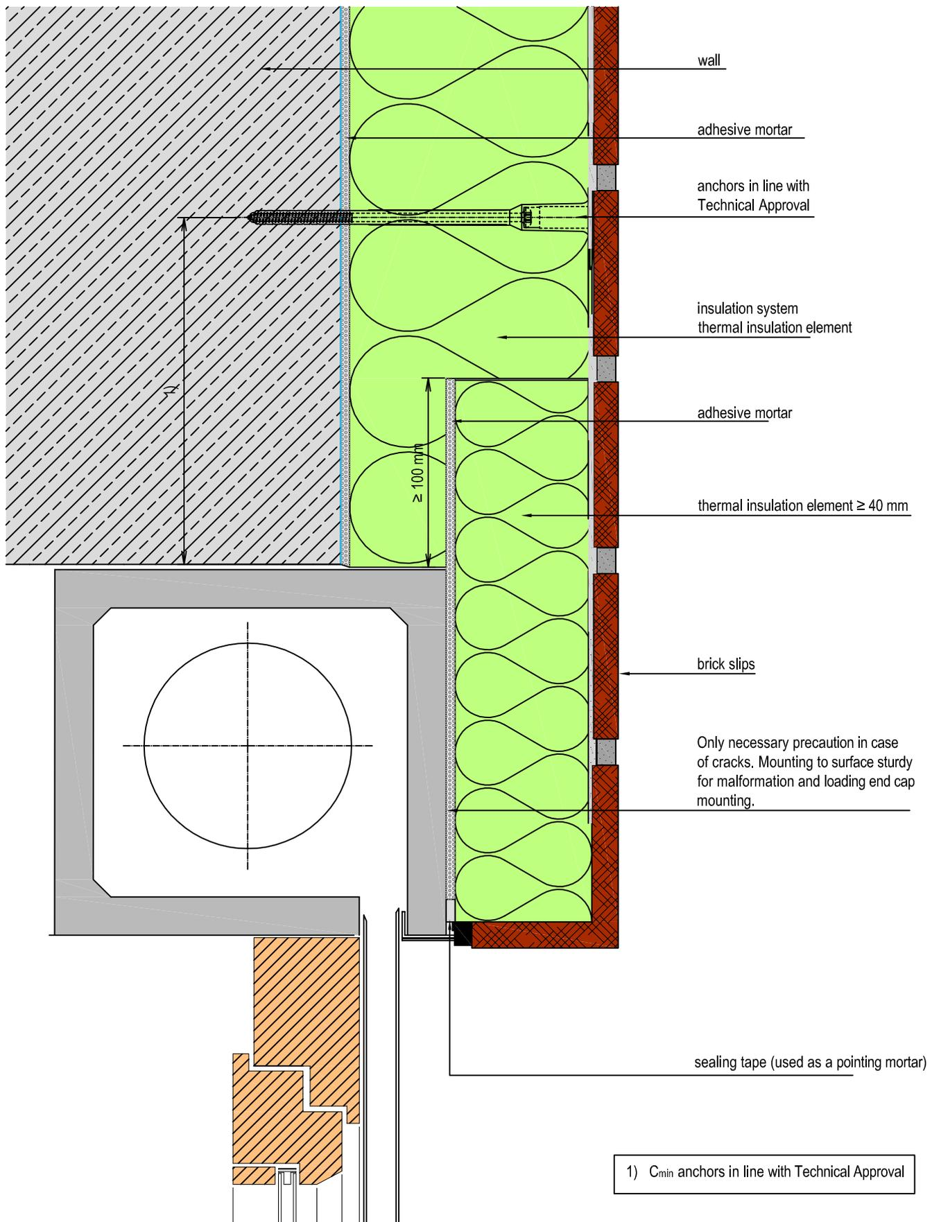
System: Klipla Insulation System with brick slips
