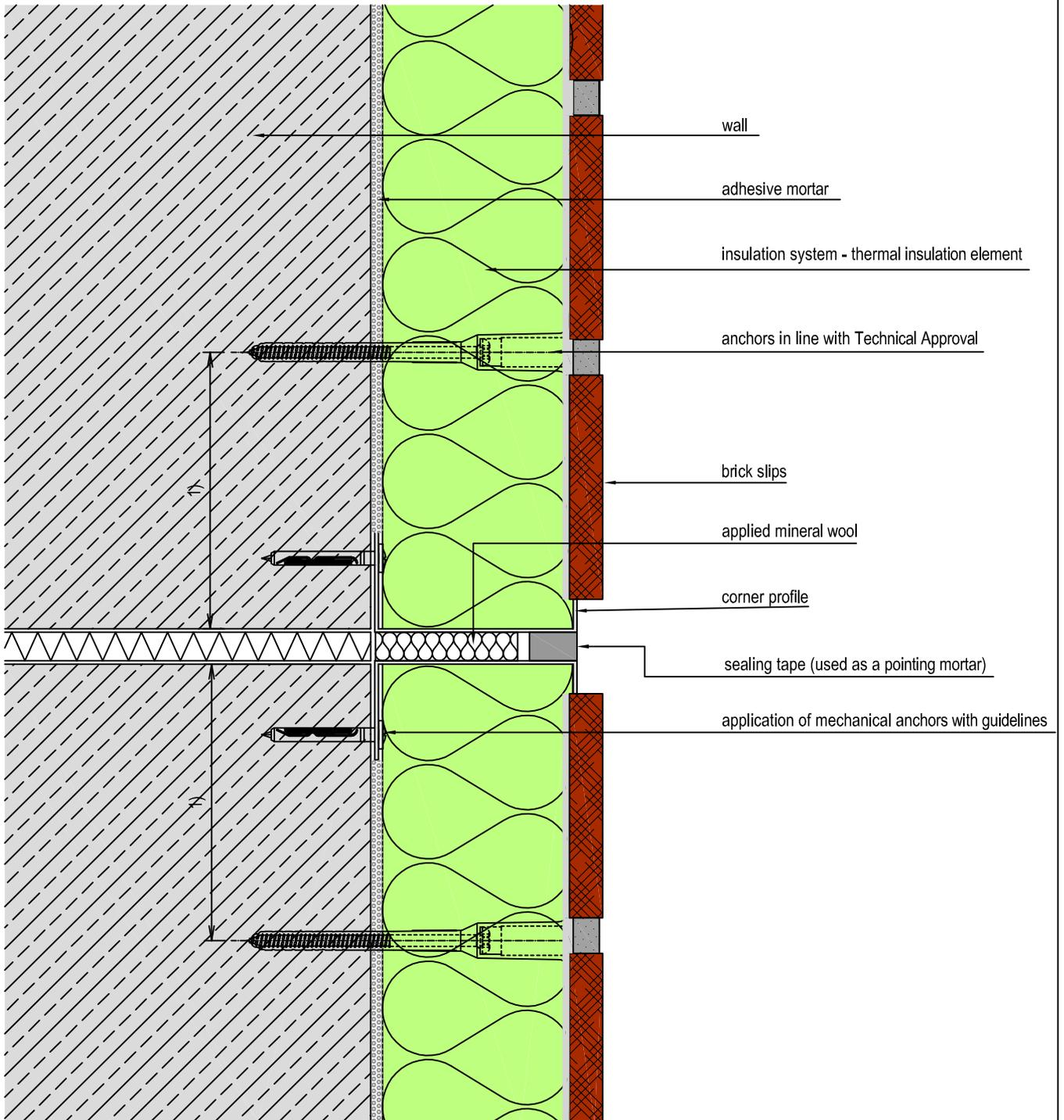
1) C<sub>min</sub> anchors in line with Technical Approval
