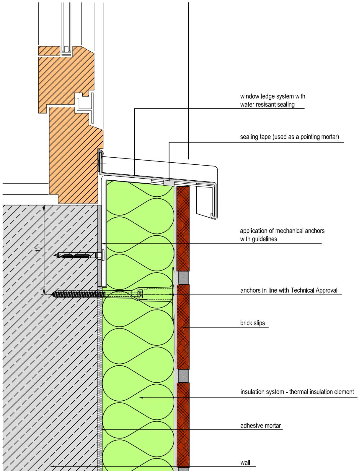
1)  $C_{min}$  anchors in line with Technical Approval
