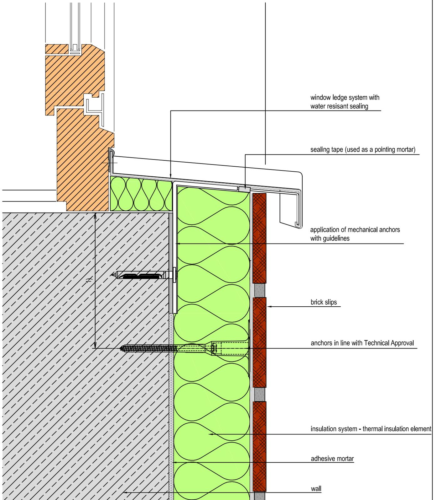
1)  $C_{min}$  anchors in line with Technical Approval
