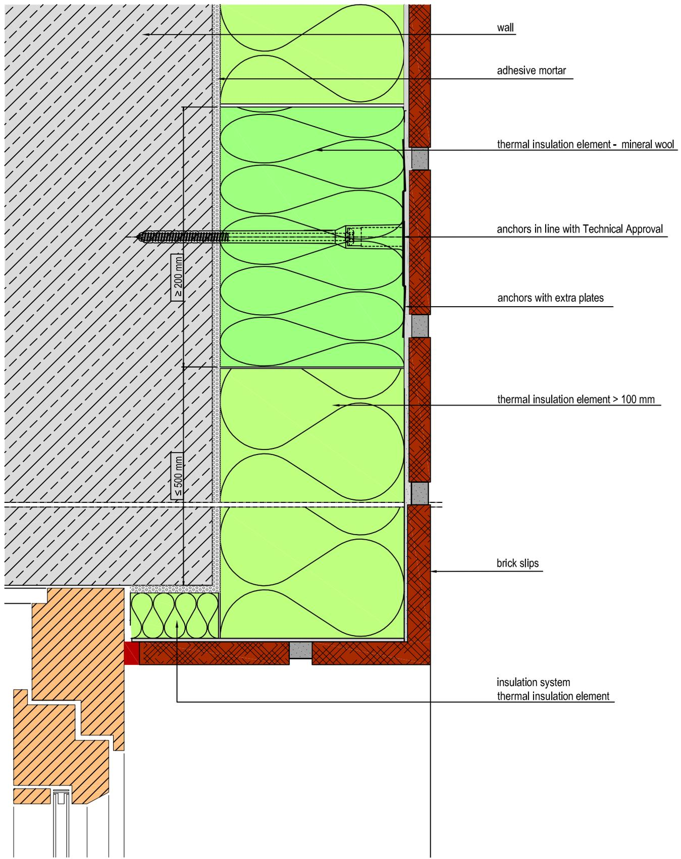
System: Klipla Insulation System with brick slips
