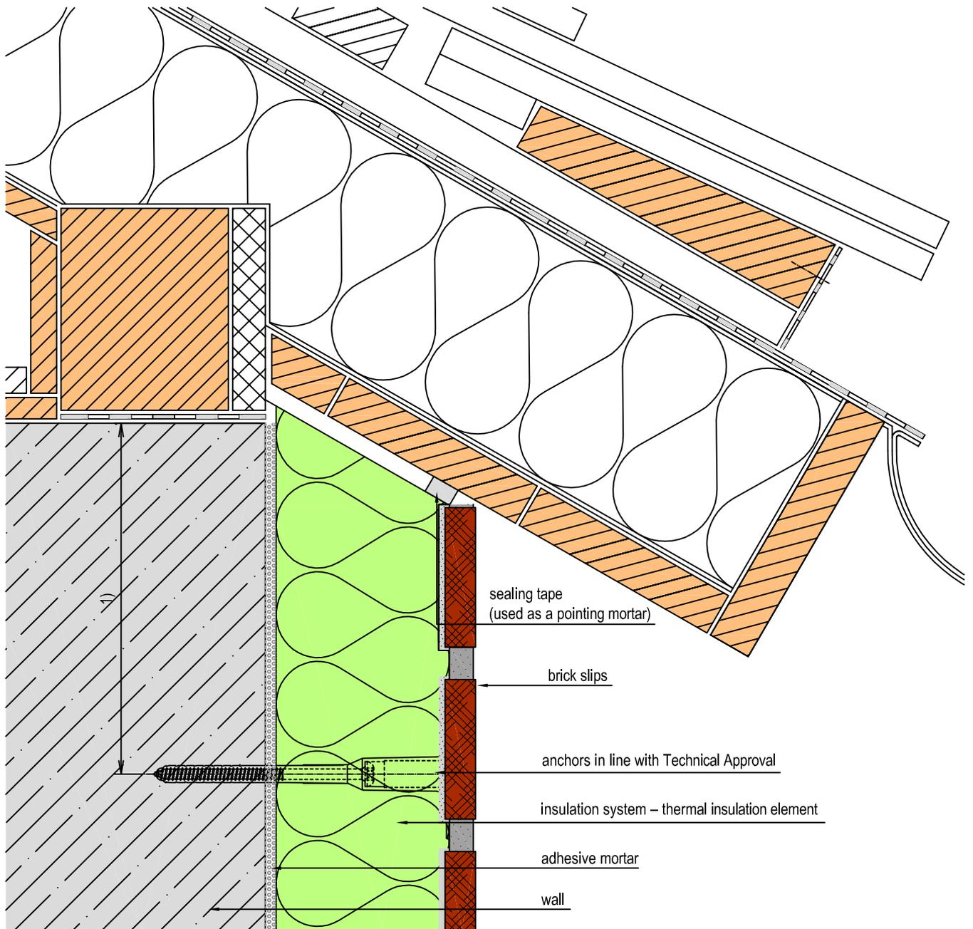
1)  $C_{min}$  anchors in line with Technical Approval
