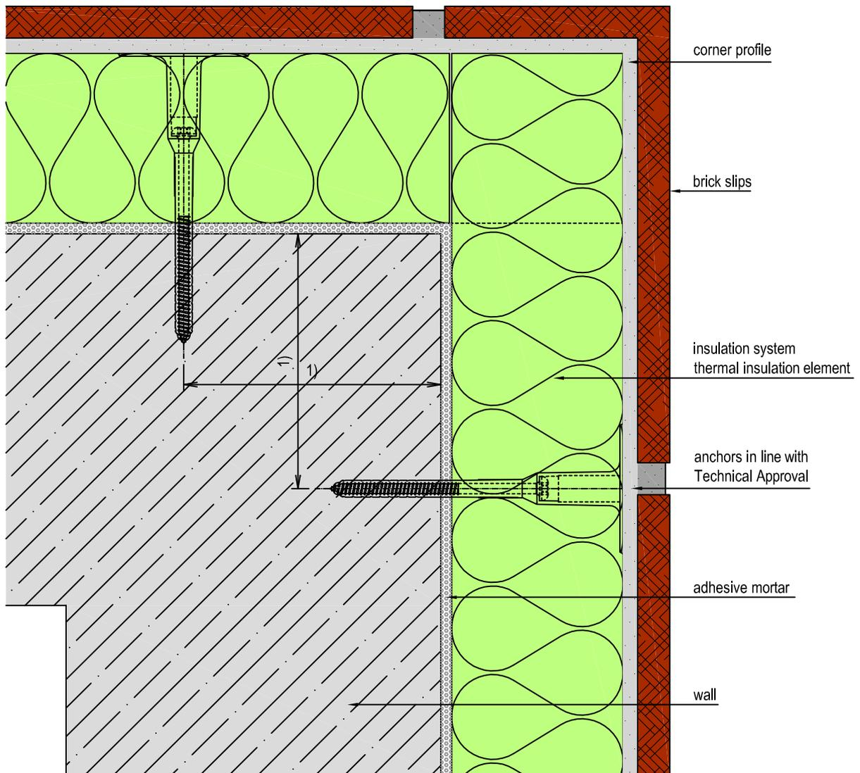
1)  $c_{min}$  anchors in line with technical approval
